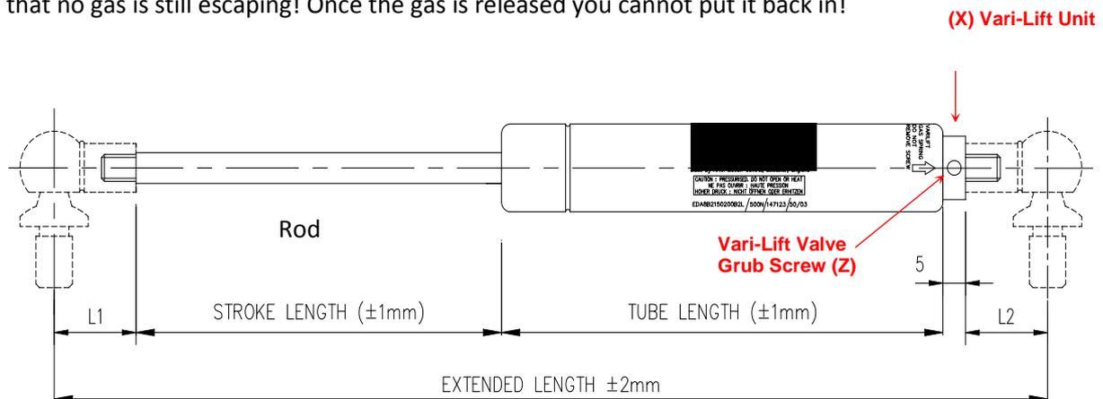
Repeat the process gently releasing a small amount of gas at a time until the required lifting action is achieved. If using two gas springs on the application (which is recommended) then repeat the above process on each spring in turn (alternate between both springs).
